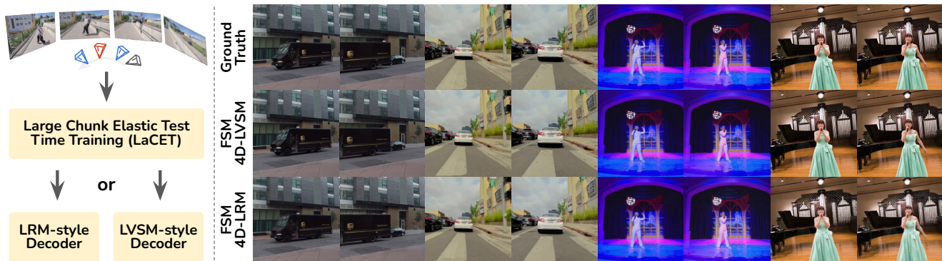
Figure 1. Fast Spatial Memory (FSM) is an efficient, scalable 4D reconstruction model that learns spatiotemporal representations from long sequences to render novel views at novel times. The model is powered by Large Chunk Elastic Test-Time Training (LaCET) blocks and is compatible with a range of rendering decoders, including LRM-style and LVSM-style decoders.
